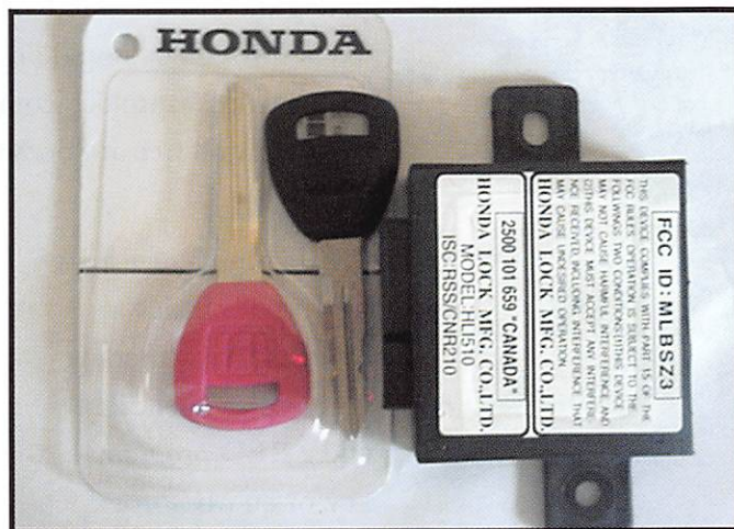
3. The Honda Type 1 system is probably the most difficult Honda system with which to work. Generating new keys requires a new module, a RED program key and an accompanying set of programmed keys.
